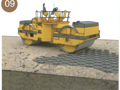
Compact GEOCELL filled with the filler using roller or compactor
